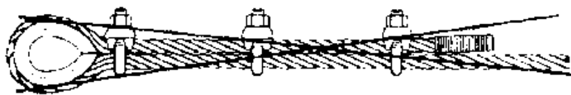
Incorrect method of fitting wire rope grips
