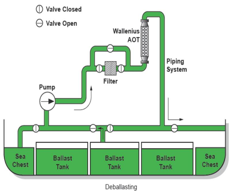
Ballast water passes through the AOT unit, but in this instance, the filter is bypassed to avoid contamination at the deballasting site.
