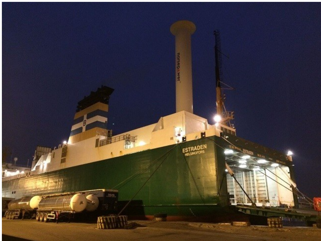
Slika 7 Brod s kružnim jedrom (preuzeto: https://www.theengineer.co.uk/rotor-sail-puts-new-spin-on-flettner-rotor/ )
