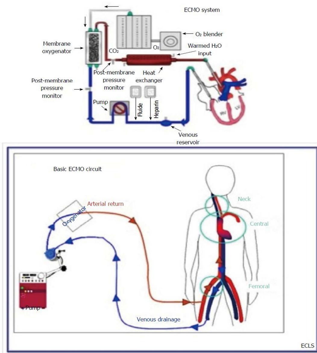
slika 1: Konfiguracija ECMO uređaja. Izvor: <https://www.wjgnet.com/2218-6255/full/v5/i2/WJR-5-78-g002.htm>
