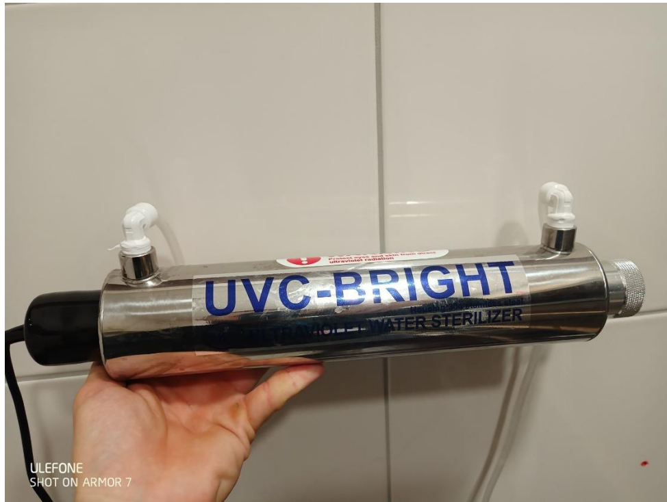
Figure 9. UV sterilizer used in the experiment (source: M. Prečanica).
