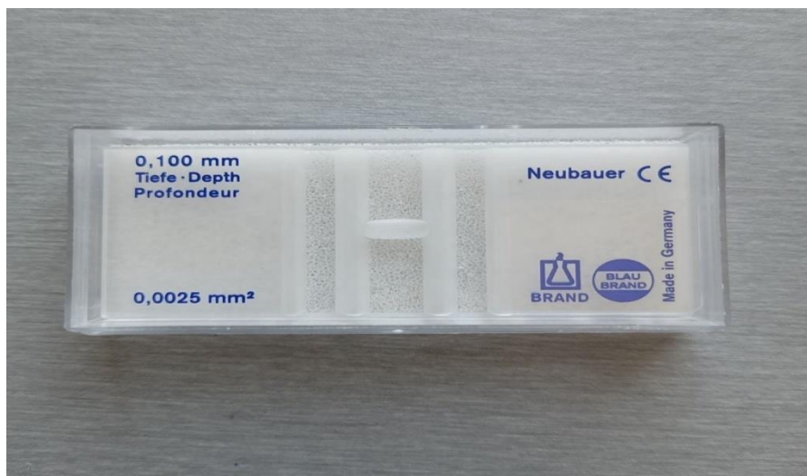
Figure 14. Neubauer chamber for counting algae cells (source: M. Prečanica).
