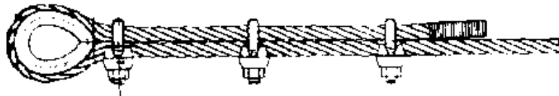
Correct method of fitting wire rope grips
