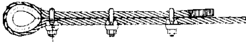
Correct method of fitting wire rope grips
