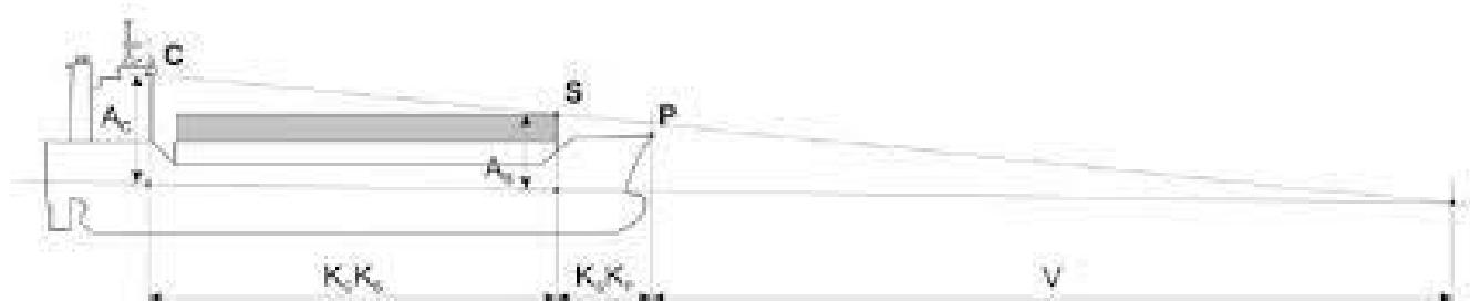
*Figure 3.1. Distances used for calculating the bridge visibility*
