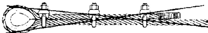
***Incorrect method of fitting wire rope grips***
