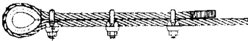
***Correct method of fitting wire rope grips***
