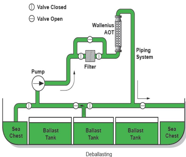
Ballast water passes through the AOT unit, but in this instance, the filter is bypassed to avoid contamination at the deballasting site.
