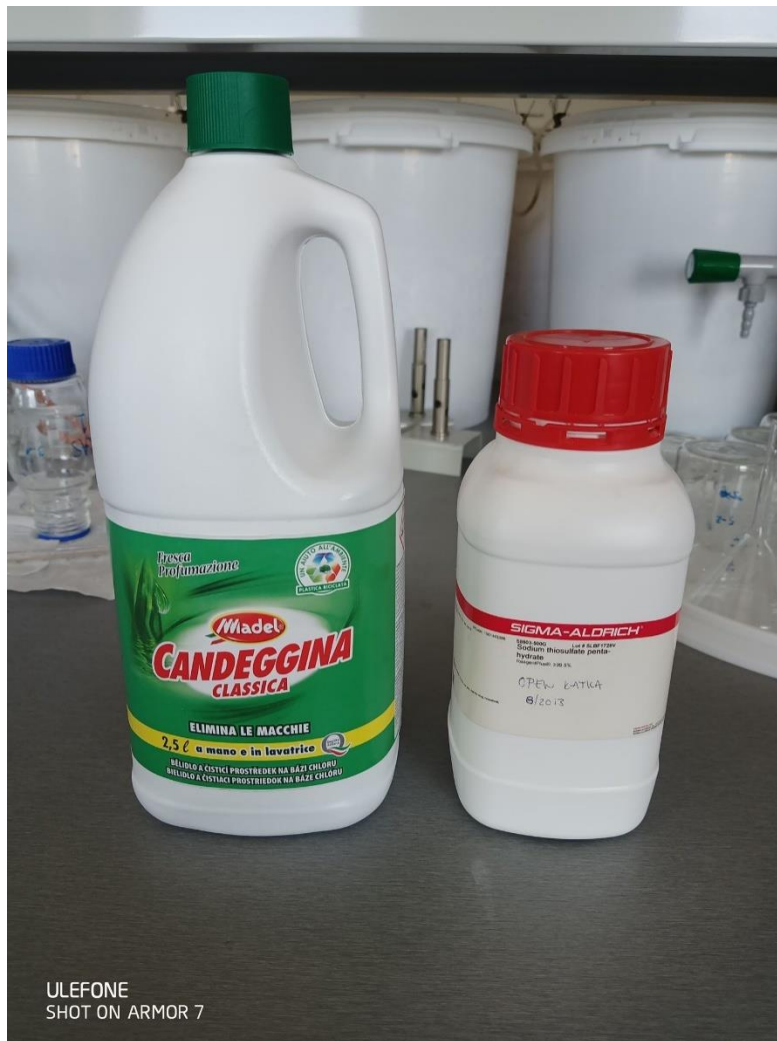
Figure 10. Bleach with 5 % of active chlorine that is used for disinfection and sodium thiosulfate pentahydrate that is used for neutralization of chlorine (source: M. Prečanica).
