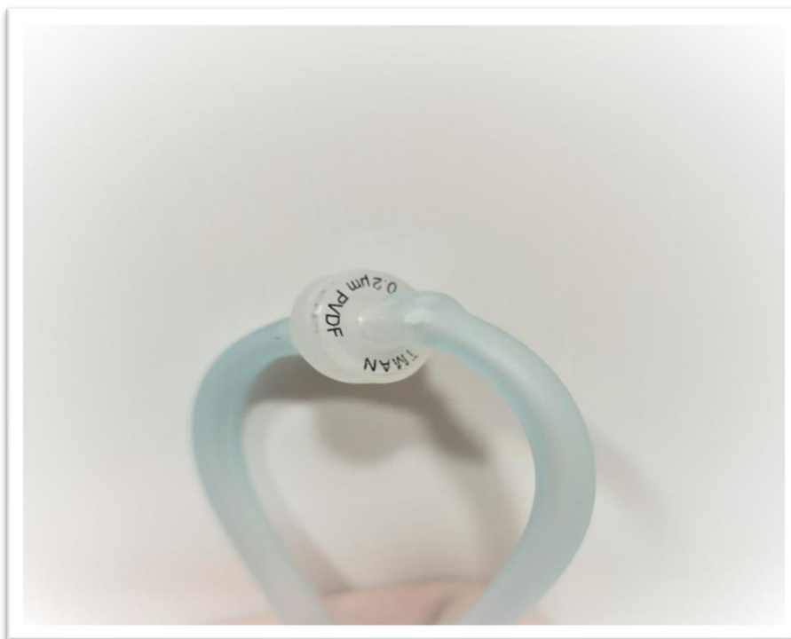
Figure 12. Whatman filter used for air filtration before entering Erlenmeyer flasks (source: M. Prečanica).
