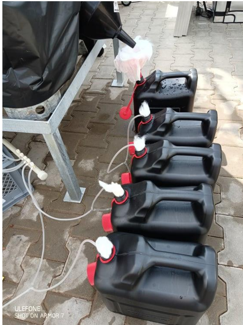
Figure 6. Black canisters used for mechanical filtration of wastewater used in the experiment (source: M. Prečanica).
