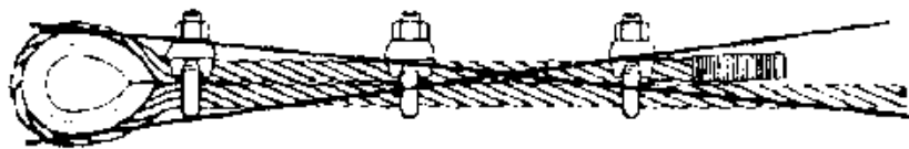
Incorrect method of fitting wire rope grips
