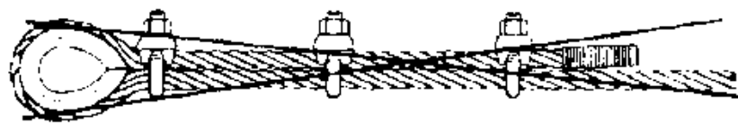
Incorrect method of fitting wire rope grips
