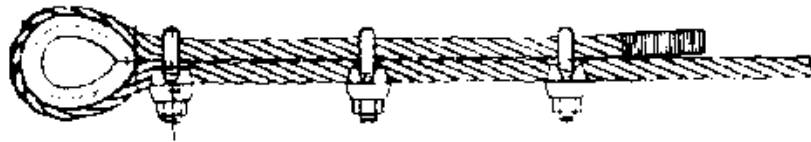
Correct method of fitting wire rope grips
