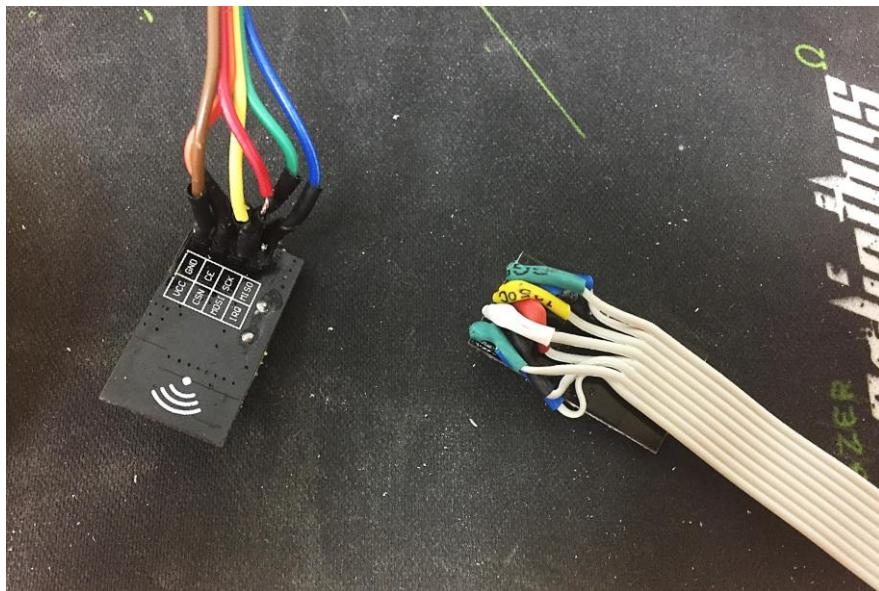
*Slika 7.8 HC-05 bluetooth modul i NRF2401 radio modul*
