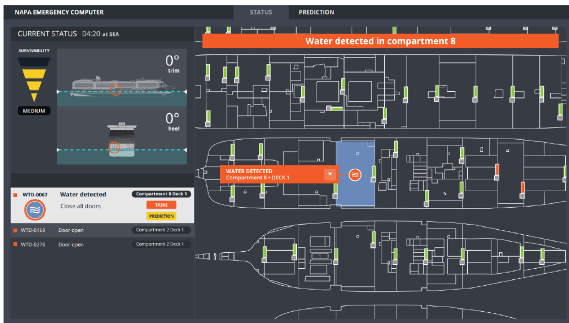
NAPA Emergency Computer - Status Monitoring
