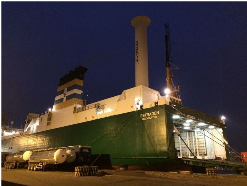
Slika 7 Brod s kružnim jedrom (preuzeto: https://www.theengineer.co.uk/rotor-sail-puts-new-spin-on-flettner-rotor/ )
