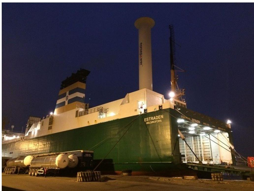
Slika 7 Brod s kružnim jedrom (preuzeto: <https://www.theengineer.co.uk/rotor-sail-puts-new-spin-on-flettner-rotor/>)
